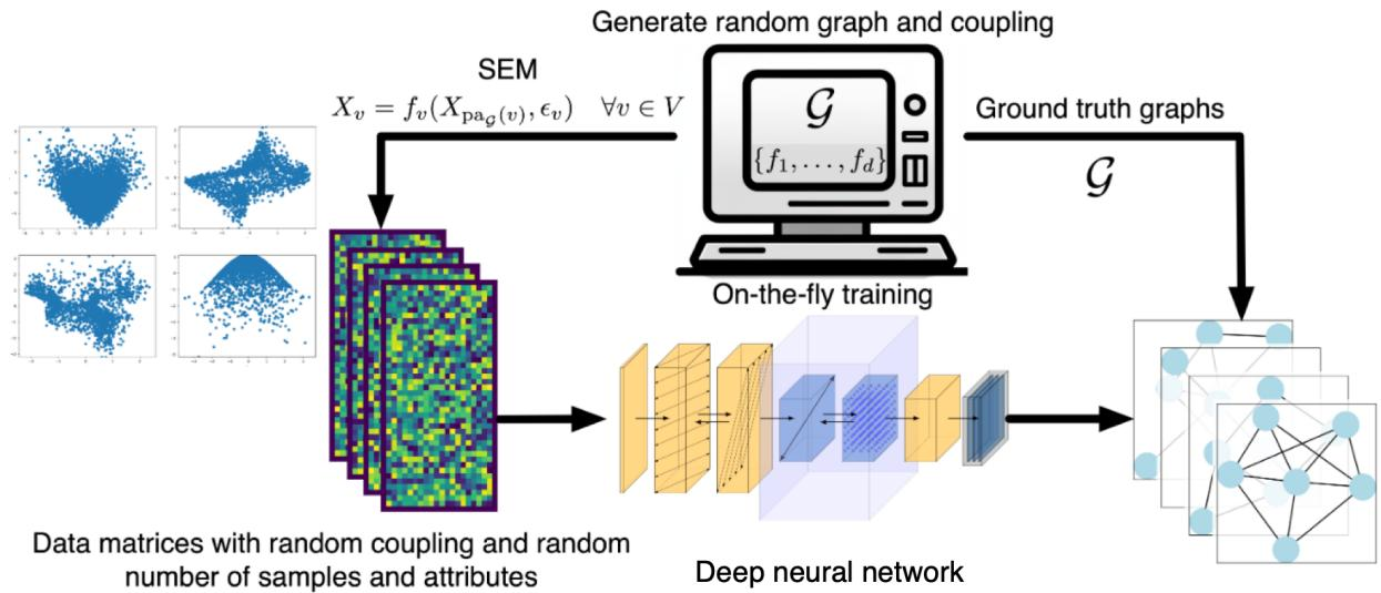
Supervised causal learning approach. We generate synthetic training data by first creating random ground-truth graphs. Then, observational data matrices are generated using SEMs given the ground-truth graphs. A mapping from observational data to the graph structure is learned via a deep neural network. Image from Froehlich and Koepll [2024].
